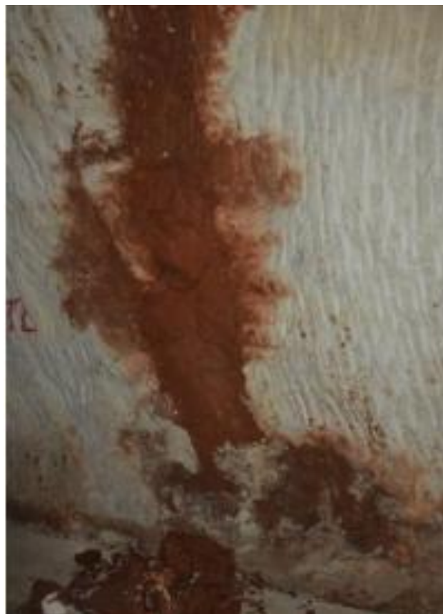
Figure 2.55: Weathered sub vertical fracture zone with terra rossa and calcite concretions
