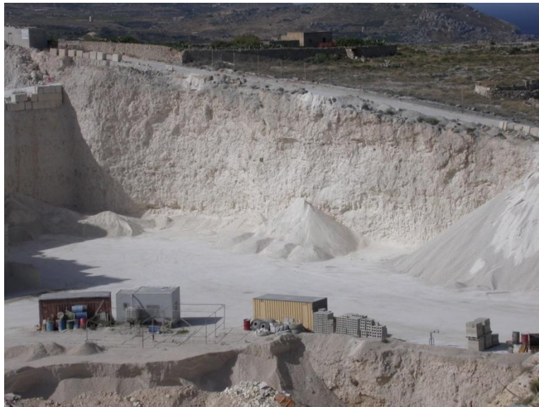
Figure 2.66: Operational Hard stone quarry in the Upper Coralline Limestone formation at Mellieha Ridge
